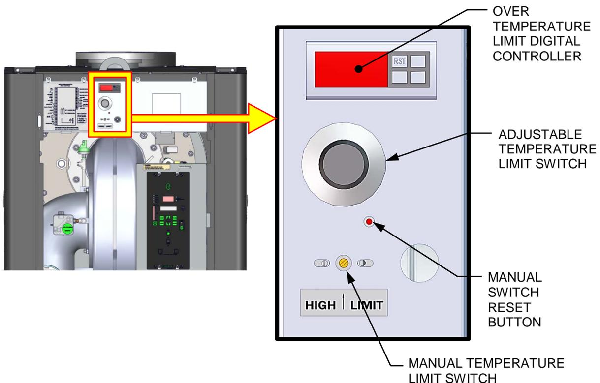
*Figure 5-4: Temperature Limit Switch Location*
