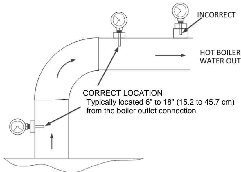
**Figure 2-7: Pressure/Temperature Gauge Installation Location**
