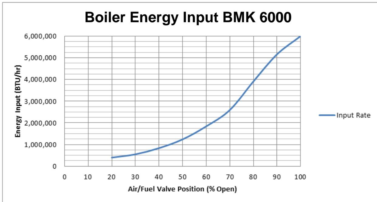
Figure 3-6: Relationship Between BMK 6000 Air/Fuel Valve Position and Energy Input
