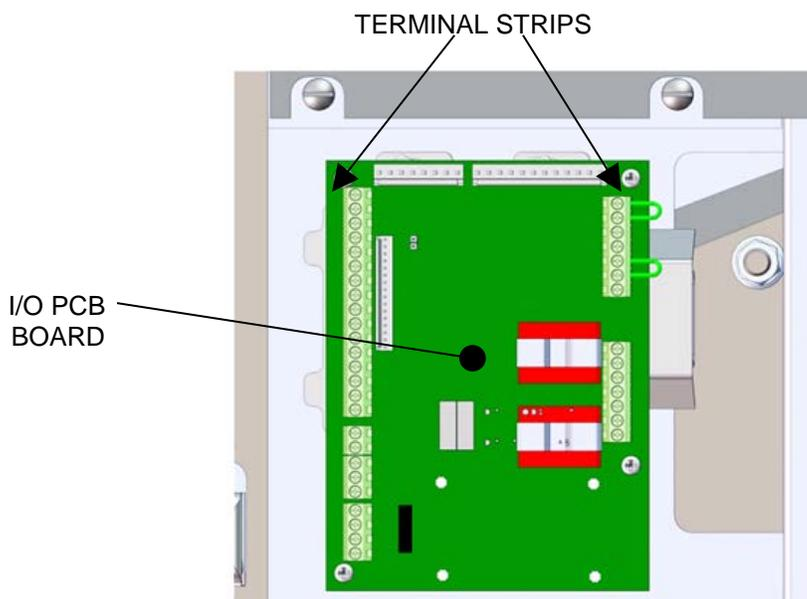
*Figure 2-14b: Input/Output (I/O) Box Interior*
