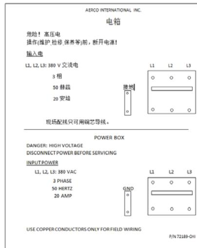
**Figure 2-13: Power Box Cover Label (P/N 72189)**
