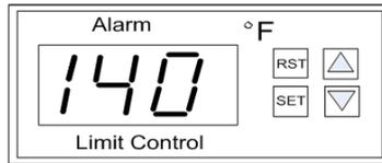
Figure 4-5: Digital Over-Temperature Alarm Switch Front Panel
