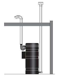
Sealed combustion with roof terminations
