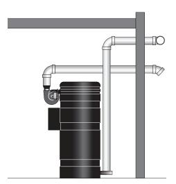
Sealed combustion with sidewall terminations
